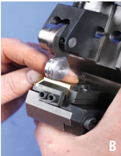
Preset the dimensions on a workbench, setting the distance between the roll and the tool.
